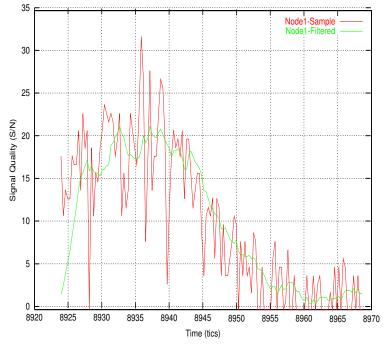
Figure 7: Sample vs. Filtered Signal Quality
