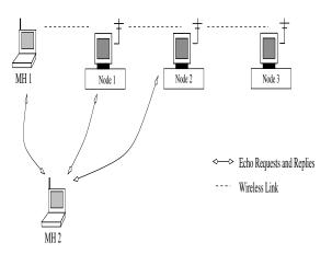
Figure 5: Measuring Signal Quality
