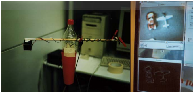
Figure 10 – Conceptual design of the tethered robot with propulsion configuration of pulling unit to produce the swing control and two counter rotating units at the tail to produce preloaded yaw control.
