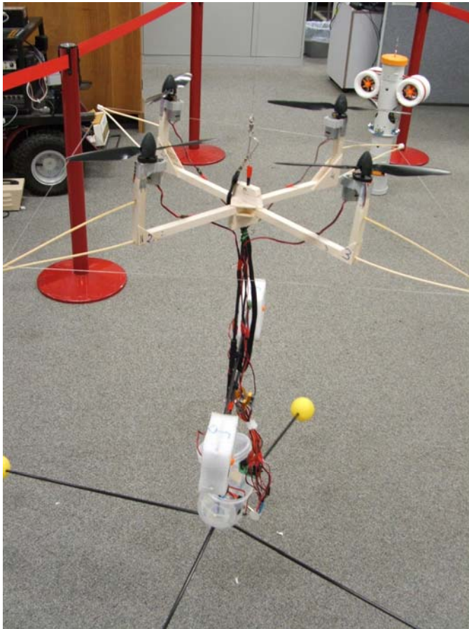
Figure 17 – We investigated the issues of controllability and computer interfaces using this setup. We tested hovering while being tethered to the lab ceiling and also as a free body.
