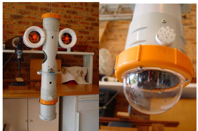
Figure 13 – The prototype of the tethered robot (left) and a close up on the dome (right) which accommodate a wireless camera on pan & tilt unit.
