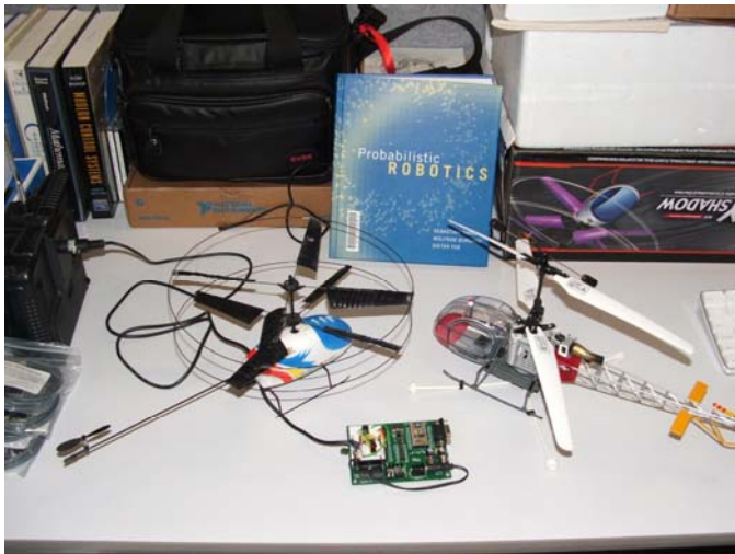
Figure 6 – RC toys used to investigate hovering & flying qualities. The Blade Runner is on the left while the Hirobo Lama on the right. In the middle is the Parallax micro used to link the RC transmitter to the computer. We use LabVIEW virtual control panel to command the toys.
