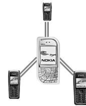
Figure 2a. A mobile 'server' configuration allows any player in the ensemble to affect sound on other phones.
