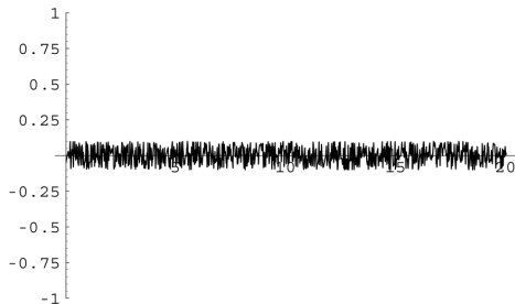
Fig. 2. Simulated correlation function g(t) between the points 4P_i and power consumption C_i(t) when d_{\ell-2} = 1 . No peak is observed since the points 4P_i are never computed by the card.
