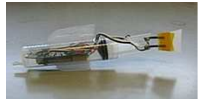
Figure 1: Prototype Robotic fish with polypyrrole tri-layer actuators.
