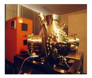
Excimer Laser Ablation System for Thin Film Deposition
