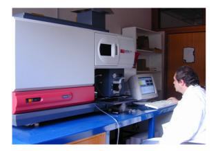
ICP-OES, Vista Simultaneous Axial Spectrometer
