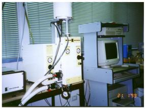
Simultaneous DTA/TGA to 1700°C
