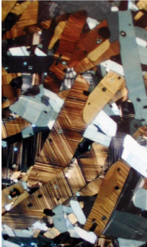
Figure 1-Photomicrograph of superconducting \text{YBa}_2\text{Cu}_3\text{O}_{7-x} , magnified 150x, to show its complex Perovskite type crystal structure. [1]
