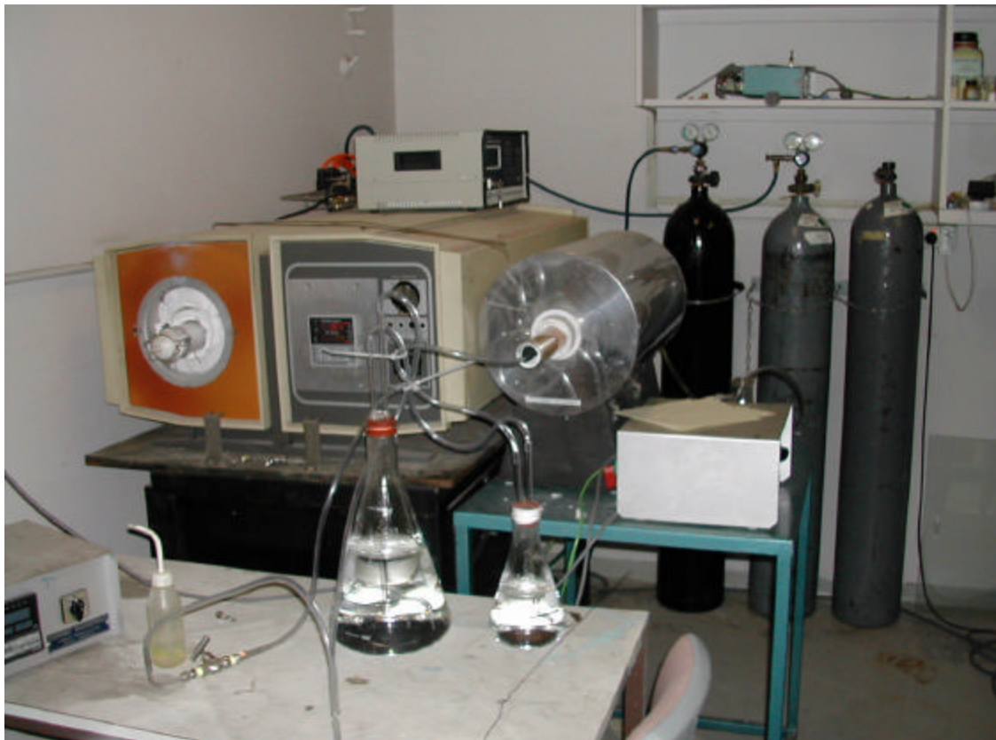
Figure 2- The laboratory furnace used for heating the samples to allow the growth of YBCO thin films
